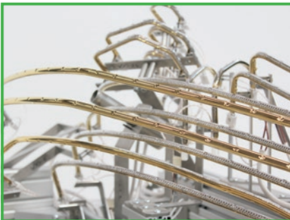
134 kW fast medium tungsten heating platen fitted with custom built curved quartz tungsten emitters. Used to heat plastic substrate in an automotive application.
