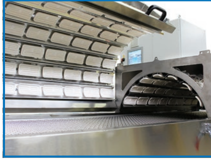
42 kW long wave ceramic conveyor oven fitted with white ceramic emitter model HTE. Used to cure foam on speaker housings.
