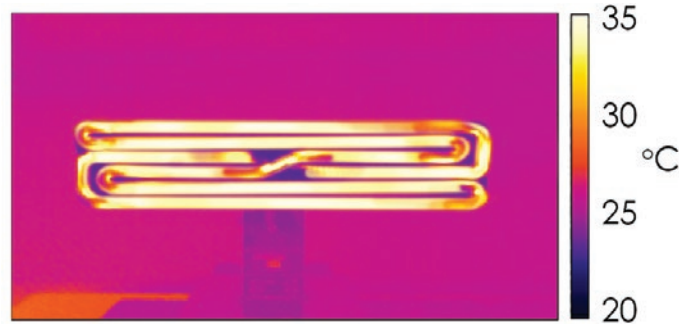
Thermal image of FTE ceramic element under test on our semi automated validation equipment
