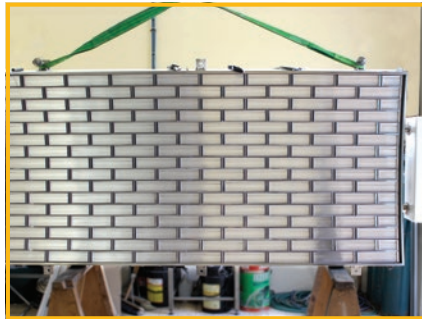
108 kW medium wave quartz heating platen fitted with quartz emitter model FQE. Used to heat PVC coating in calendaring machine.
