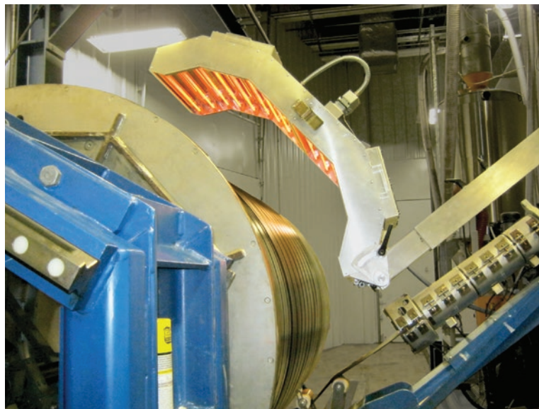
Infrared heating of billet winder. In this process, HDPE is extruded at the point of wrapping and directly wound onto a metal framed mandrel to create large diameter pipes. A 36kW Fast medium wave modular infrared heater is used to heat the already formed pipe shape to prepare the surface before overlaps thus ensuring a good fusion bond is made with the underlying wrap. On completion of winding, the mandrel is collapsed and retracted allowing the formed barrel or pipe to be removed. These finished forms are then used to fabricate custom parts with high integrity and minimal waste.
