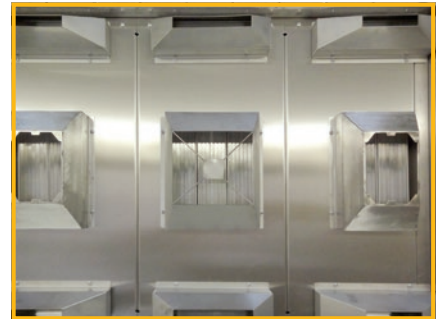
16.9 kW medium wave quartz heating platen fitted with quartz emitter model PFQE. Used to infrared weld plastic components.
