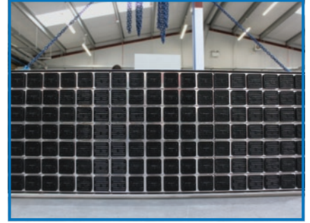
75.6 kW long wave ceramic heating platen fitted with black ceramic hollow emitter model SFEH. Used to pre-heat carbon fibre fabric.
