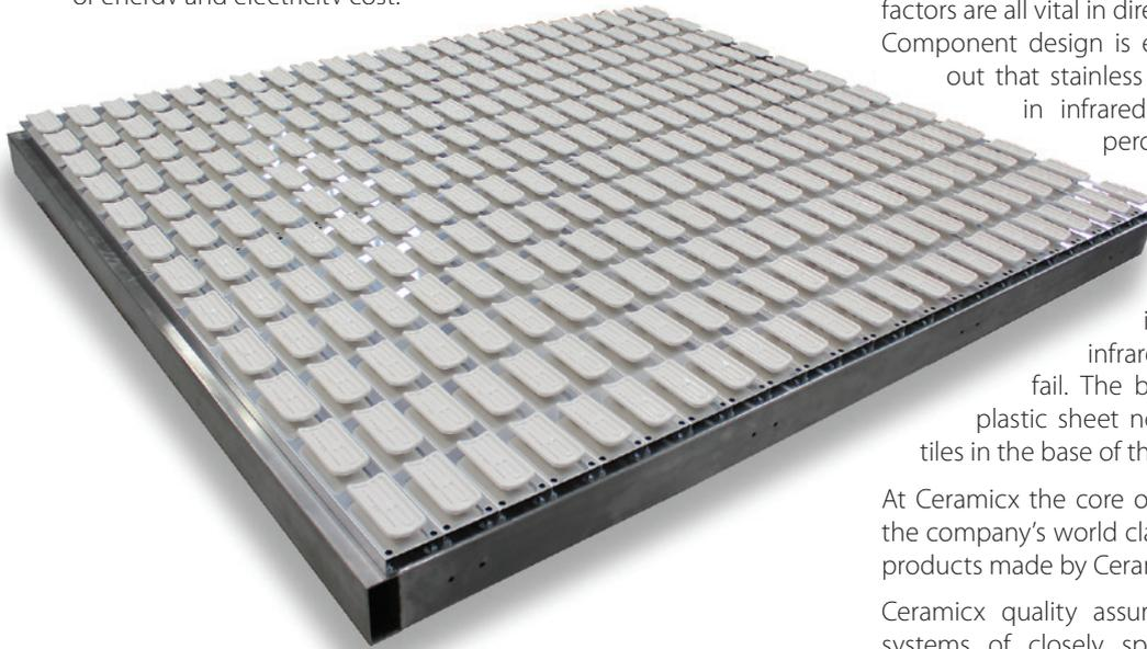
*Infrared (IR)-based replacement heating platen part of a top and bottom system with 276 ceramic heaters in 18 zones.*
