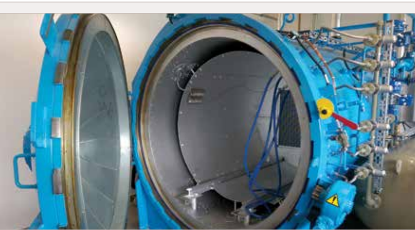
The autoclave at Belfast Met is capable of 250°C and 10 bar pressure and is used to manufacture high quality thermoset composites. The Vector machine is aiming to reduce capital costs, energy consumption, cycle time, floorspace and facilities integration costs associated with such autoclaves.
