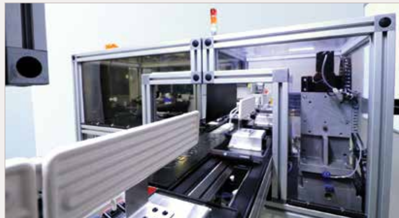
The CIRCLE ( Ceramicx Infrared Characterisation Laboratory Equipment ) test platform has modular parallel test stations, each station has a dedicated controller with power, air, communication and IO connection. The stations are connected over a network and co-ordinated by a central computer.
