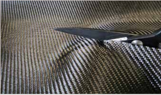
Cutting Carbon – Dry carbon fibre cloth can suffer weave distortion during handling or high pressure resin injection in processes such as RTM or RTI. Pre-forming with Ceramicx IR machines prior to injection can reduce weave distortion and greatly enhance quality in aerospace composites.
